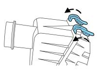
5. Remove the air filter element from the air filter housing.
